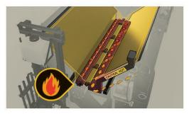
**Radiant oil heating** maintains asphalt and tack tank temperature with superior consistency and uniformity.
