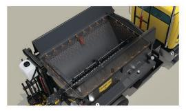
Release agent spray bar coats hopper to prevent asphalt from sticking, so crews don't have to climb truck or enter hopper.
