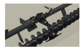
Steel auger (bottom) and anti-bridge bar (top) ensure clog-free asphalt conveyance and consistent heating.
